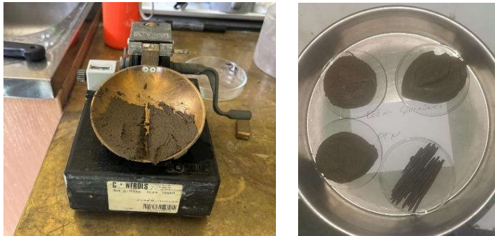
Figure 4. Laboratory determination of the liquid (left) and plasticity limit (right)
