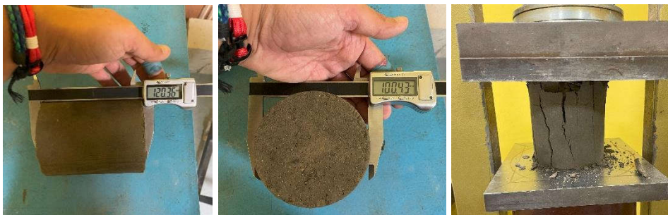
Figure 5. Laboratory investigation of UCS after 7 days of curing
