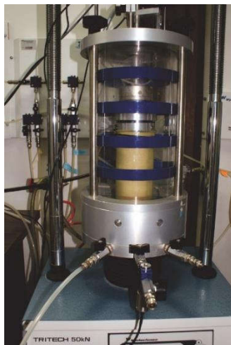
Figure 2. Triaxial apparatus with soil specimen ready for testing
