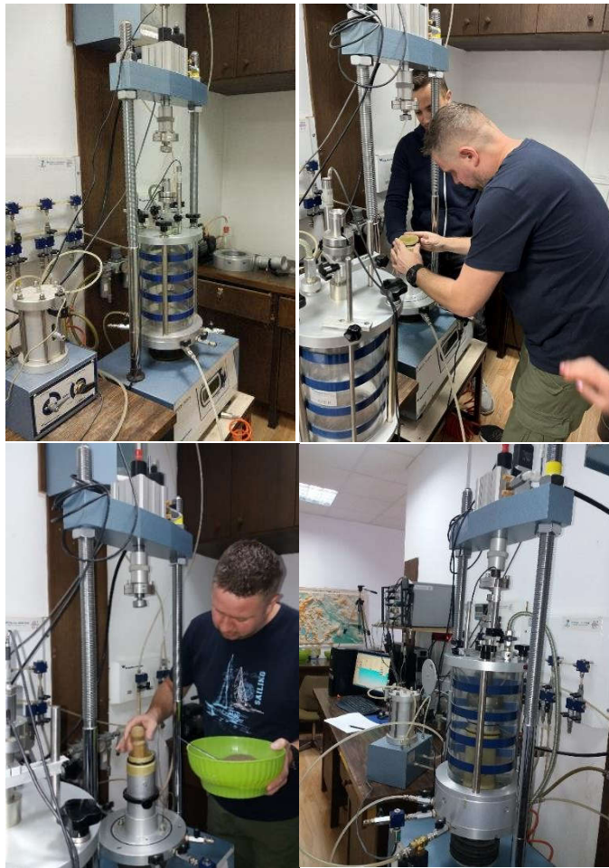
Figure 1. Triaxial apparatus - preparation of a sample for testing
