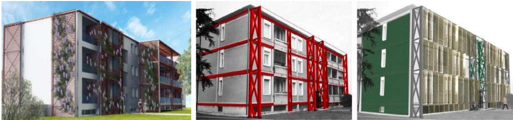
Figure 3. Application of a steel exoskeleton wall system for integrated seismic and energy retrofitting of buildings [7],[8]
