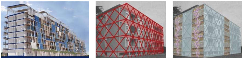
Figure 4. Application of a steel exoskeleton shall system for integrated retrofitting [8],[11]
