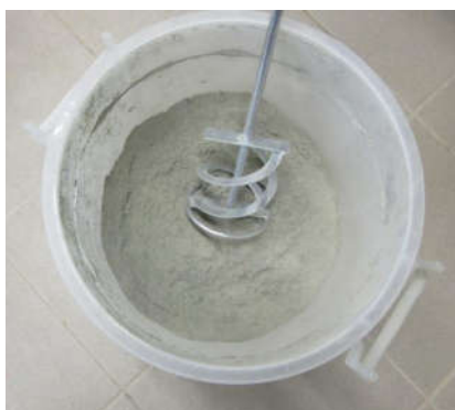
Figure 3. The container and special attachment for mixing cement and glass
