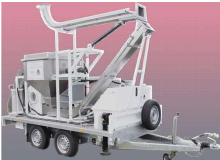
Figure 4. Machine for applications of Steel Fiber Reinforced Concrete
