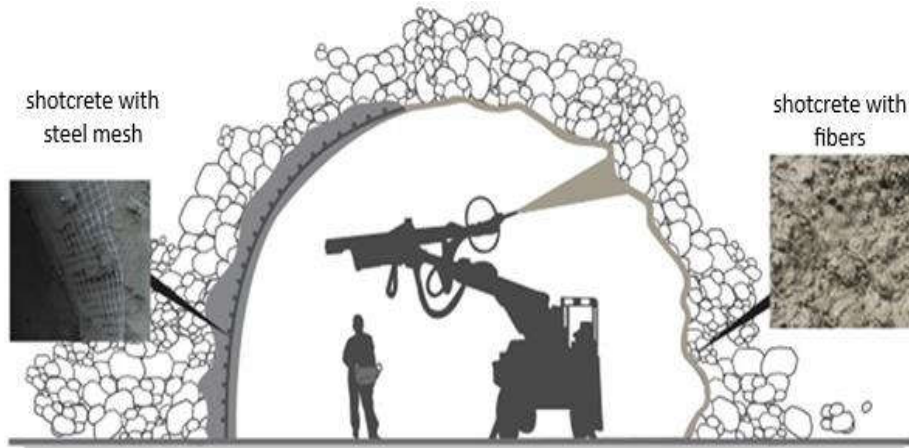
Figure 5. Shotcrete with steel mesh and with fibers
