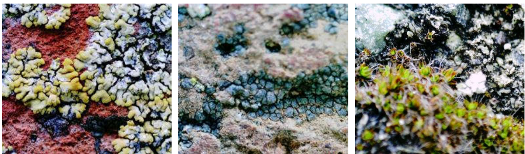
Figure 7. Different types of lichens present on the facade surfaces (images from a digital microscope with 40x magnification), [3]
