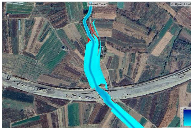
Figure 10. Extent of flooded area without and with the temporary crossing installed, Q_j=19.9 \text{ m}^3/\text{s} .
