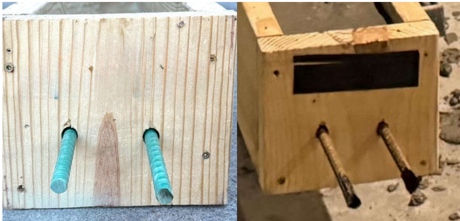
Figure 1. Beam Cross Section a) Fiberglass #4 as reinforcement b) Steel Rebar #4 [7]
