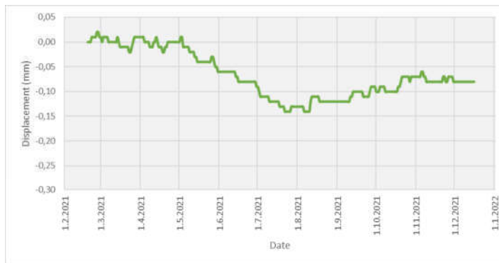
Figure 12. The diagram of crack behavior (deformer D-4V)
