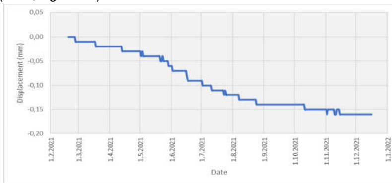
Figure 10. The diagram of crack behavior (deformeter D-4R)
