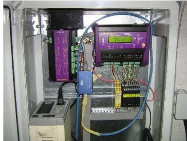
Figure 7. Layout of the measurement cabinet with data logger and accompanying equipment
