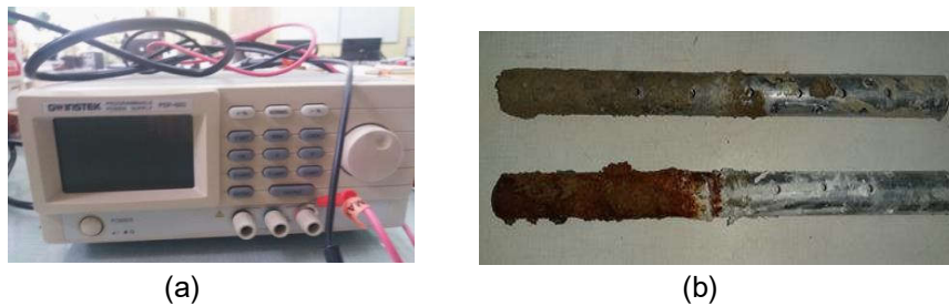
Figure 2. Direct current power supply DC (a) and corroded electrodes (b)
